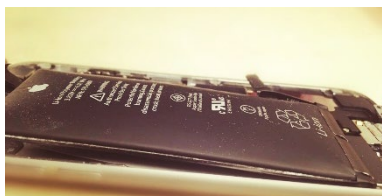
Figure 1: Swollen lithium-ion accumulator (source: SSHE)
